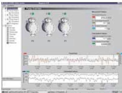
Figure 3: Pump status and status of each pumphead, as "traffic signals"
